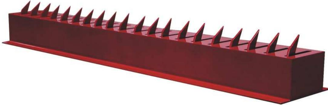
The traffic controller is a heavy duty in-ground “Directional Enforcer”. It allows traffic in one direction only. It can be used as a free entrance or exit to your parking facility. It can be used to enforce one-way traffic in such drive-through areas as hotels, banks, commuter stations, etc. The Model 200-1 is 72" wide and includes twenty cut-steel blade teeth.
