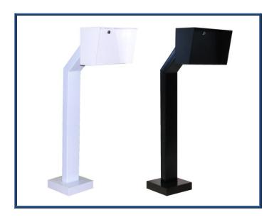
These housings are typically used to install card readers or intercoms at drive-up and pedestrian access points. The Model 306-6 pedestal is 36" tall and made of 2" X 4" rectangular steel tubing with an 8" X 8" base plate. A steel base plate cover is provided to conceal the mounting hardware. Housings are 8" tall X 12" wide with cam lock and removable "tilt-in" panel design. There is 2.5" depth behind the removable panel. Model H081206 housing is also available without a pedestal.
